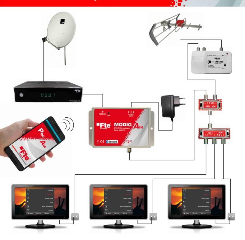
In the example the MODIG AIR is receiving signal from the HDMI output of a High Definition satellite receiver and modulating it in a terrestrial RF output channel. The DVB-T output channel is mixed with the rest of the channels of the installation with an inverted TER 2 splitter, being able to be tuned in all the TV sets. The MODIG AIR programming is done through a mobile phone or tablet via Bluetooth with the free application Fte Pro Air.
